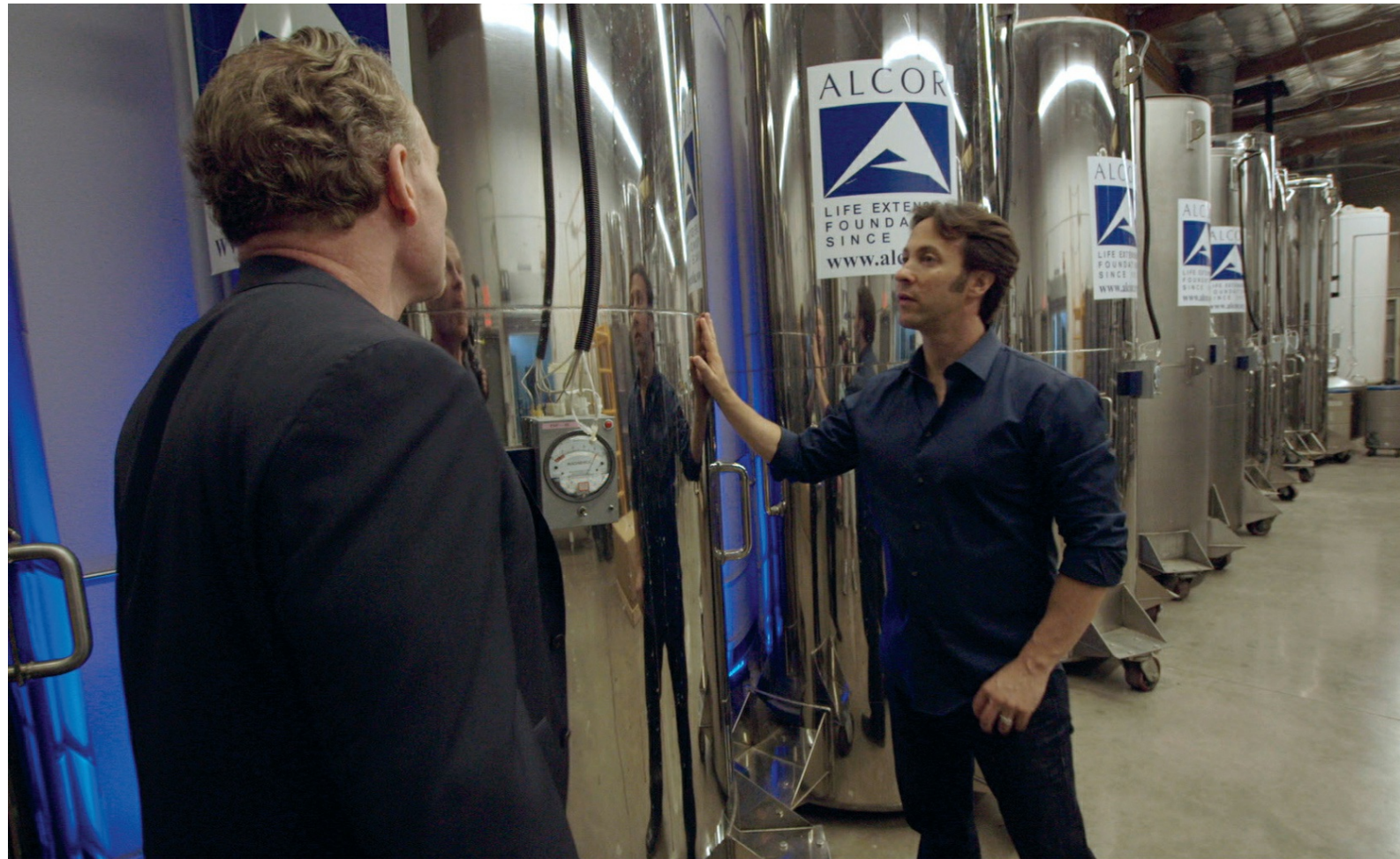
Each of these dewars stores four bodies and up to five heads, all stored at -196^{\circ}\text{C} .
